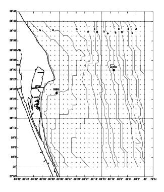
Figure 2. 2.775 km wave model grid with depth contours in meters.
