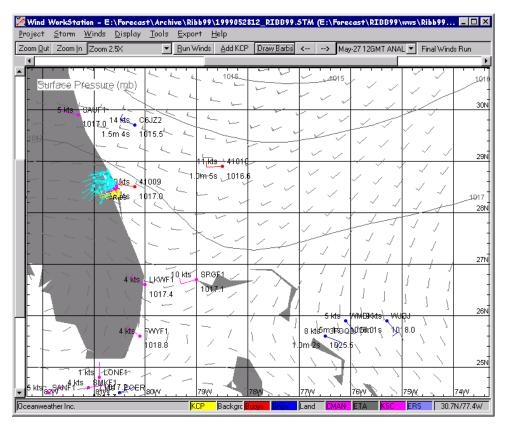
Figure 3. WWS display showing gridded AVN and ETA winds, contoured AVN pressures with *in situ* data from buoys, ships, CMAN Stations, and KSC tower winds.
